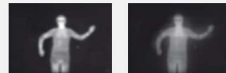
The Fresnel lenses used in Bosch's patented Tri-Focus optics produce better image quality (left) than the mirror lenses of traditional systems (right).
