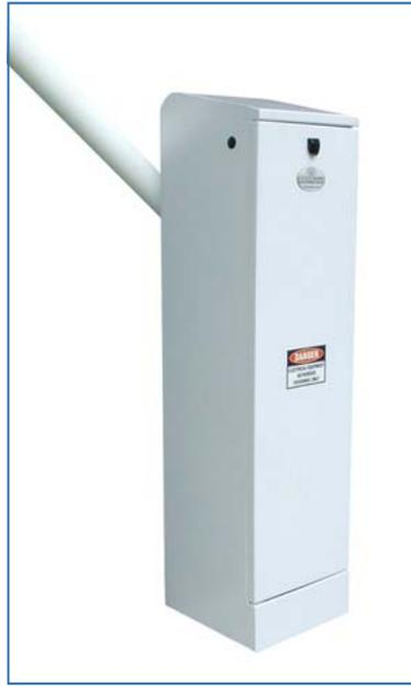
The Sector is powered by a custom built 12vdc motor and gearbox which is rated for up to 3000 operations per day with a life cycle of 5 Million operations. Variable speed on opening and closing (standard is 3 seconds) combined with damping in both end positions, ensures smooth operation and prolongs the life of the Sector.
